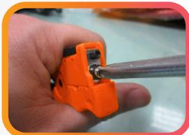
**Step 3.** Insert the fiber cable into the groove and pull the cable to slit as needed.
