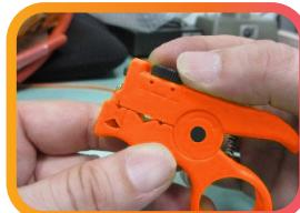
**Step 2.** Insert the fiber optic cable into the desired groove and spin the TCCPS around the cable. Dress cable as needed.
