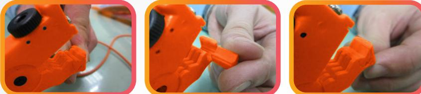
**Step 2.** If necessary, adjust the slitting blade height.
