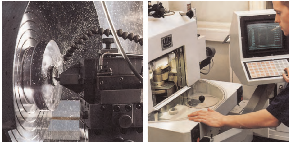
Figure 28.4 LEFT: Diamond turning machine; RIGHT: Lens polishing
