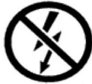
The Teledyne Test Tools Rogowski probes do not provide protection of the user from electric shock whilst applying or removing the probe from HAZARDOUS LIVE conductors. Additional protective means are necessary to avoid electric shock from HAZARDOUS LIVE conductors which cannot be de-energised.
