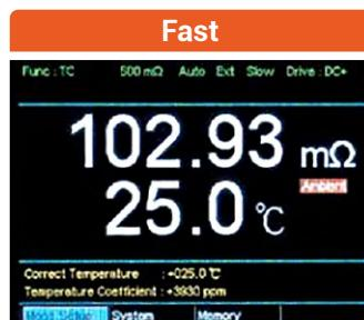
T3MIL series offers Fast (60 readings per second) and Slow (10 readings per second) measurement speeds.
