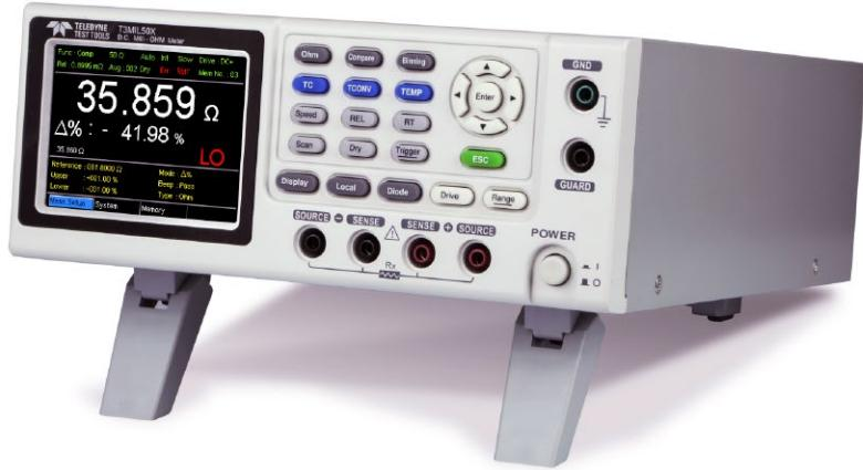
**Teledyne Test Tools introduces a brand new series of D.C. Milli-Ohm meters. The T3MIL series offers two models T3MIL50 and T3MIL50X, which features a 3.5-inch TFT display with a measurement accuracy of 0.05 %, maximum 50,000 count measurement display and sampling rate of 60 readings per second. The T3MIL series also provides four wire measurement as well as temperature measurement and temperature compensation functions to meet the requirements of low resistance measurement applications.**
