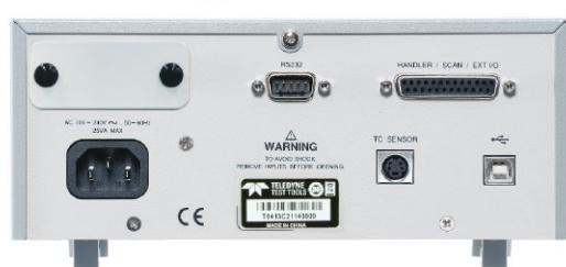
T3MIL series provides a D-sub 25-pin combined interface to control the device for various functionalities such as Handler, Scan and EXT I/O. Handler function can be used for connecting the device to a sorting machine in a production environment. Scan and EXT I/O is useful when connecting to an external switch or for an external trigger control. T3MIL series also offers remote control and data retrieval through various interfaces such as RS 232C and USB.
