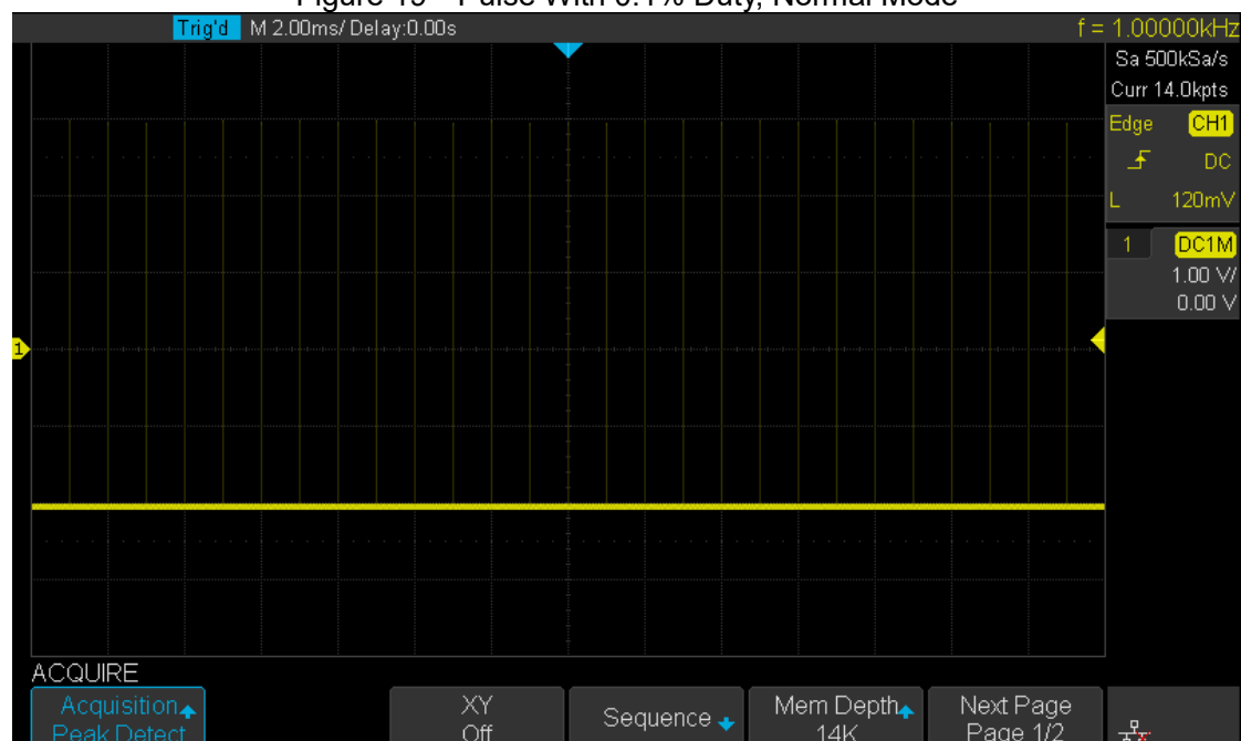
Figure 20 Pulse With 0.1% Duty, Peak Detect Mode
