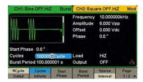
Burst mode supports 'N Cycle' and 'Gated' modes with the Burst source being configured as 'Internal', 'External'
