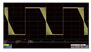
The rise/fall times can be set independently to a minimum of 8.4 ns at any frequency and to a maximum of 22.4s.
