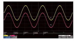
Output amplitude into a high impedance load can be as high 20 Vpp at frequencies up to 20 MHz, and 10 Vpp for frequencies greater than 20 MHz.
