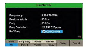
The counter functionality, accessed via the rear panel BNC, gives a DC or AC coupled counter capability from 100 mHz to 200 MHz.
