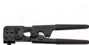
Compound-action tool crimps 10-22 AWG insulated terminals to meet or exceed MIL-SPEC pull-out tests. Built-in ratchet with safety release ensures uniform crimps every time. Compound lever-action of narrow-span handles puts more crimping power into each squeeze.
