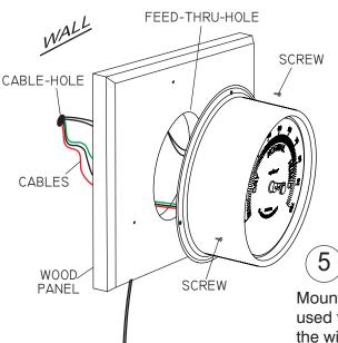
Mount the brass instrument directly over the cable hole used to route the power and sensor wires to avoid crimping the wire under the lip of the case. We recommend mounting the brass instrument on one of our pre-drilled and centered wood panels. Plug the AC adapter into a 110 VAC power outlet.
