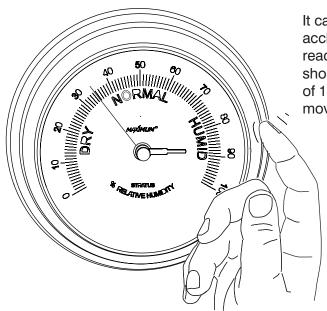
It can take 12-24 hours for the humidity sensor to acclimate to its surroundings and reflect accurate readings. Before reading your Hygrometer, you should tap the case with your finger. A tap change of 1-2% is a common occurrence with any slow moving precision meter movement.
