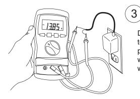
Disconnect the AC adapter from the indicator and connect it to an AC voltmeter. Plug the AC adapter back in. If working properly, the AC adapter will deliver 11.5 to 18VAC. If not working properly please contact Maximum. If the Adapter is working properly, continue to step 4.
