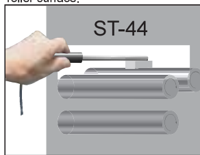
Temperature measurement of roller surface.
