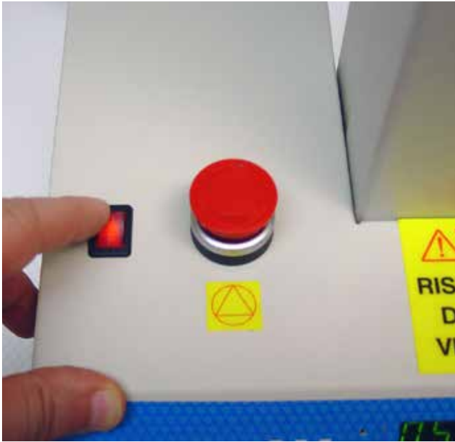
The ON/OFF switch is a 2-way switch. The switch is lighted when power is ON.
