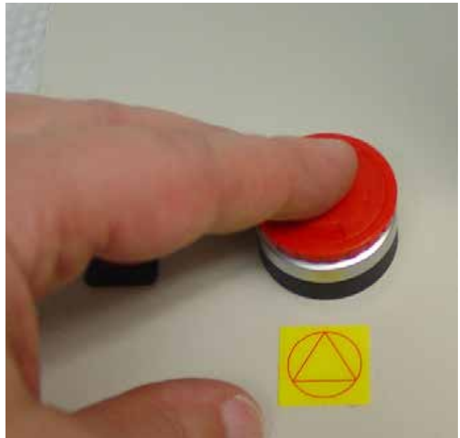
Engage the Emergency OFF switch by pressing down on the red button. To disengage the emergency switch, press and turn counter clockwise. This will release the button to its normal position.
