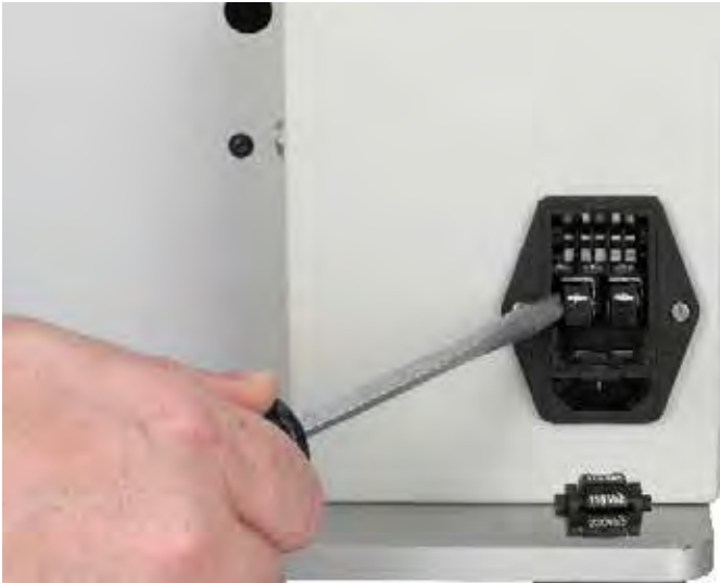
Place the side of the screwdriver next the fuse release button and apply slight pressure in the direction of the arrow.
