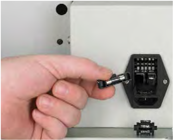
Replace the 1-Amp fuse with another 1-Amp fuse. Reinsert the Fuse Module and depress the arrow button until it locks securely.
