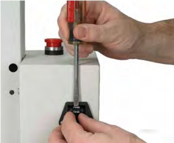
Insert screwdriver into Power Entry Module slot. Carefully apply pressure to open the module.
