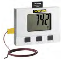
SM320 2 Channel Temperature Logger (Internal & Remote K-TC)
