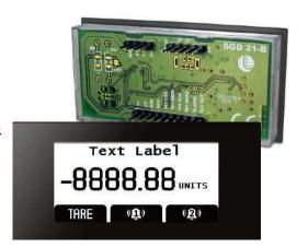
The display works with free PanelPilot B configuration software (available for Windows 7, 8 and 10) providing six analogue and digital voltmeter Apps which can then be customised to suit individual applications. Elements of each configuration that can be changed in software include custom labels, scaling and alarms. A splashscreen can be added to display on power-up.
