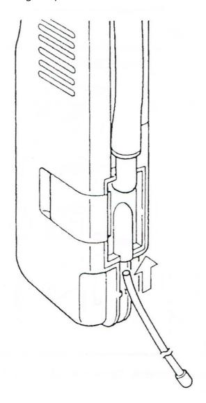
(1) Push the Nozzle into the hole located at the bottom of the Sample Chamber until it stops.
