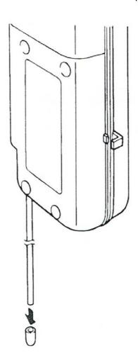
(3) Confirm that the Sample Chamber has been filled with water. If bubbles are present in the Sample Chamber, operate the Tube Pump again to refill water into the Sample Chamber.
