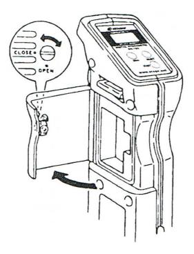
**(2)** Insert the battery as indicated, take note of the polarity.
