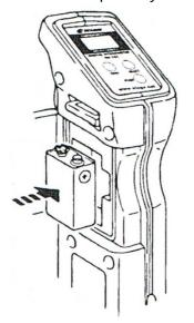
Note: The battery (006P) provided with the Unit as an accessory is to be used to check that the Unit operates properly. The battery itself is not guaranteed, and be sure to use a new battery if its voltage is low.
