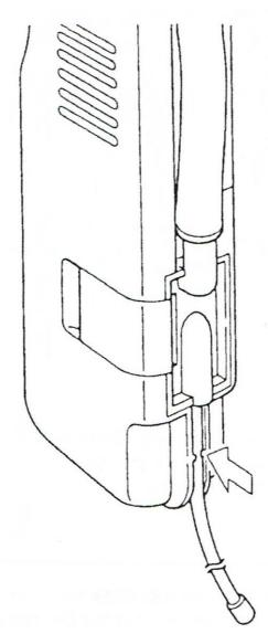
**(2)** Then, fit the nozzle into the slit by pushing with the thumb.
