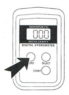
(5) Zero-Setting is now complete. Remove the Nozzle from the water and squeeze the Tube Pump to drain the water from the Sample Chamber.
