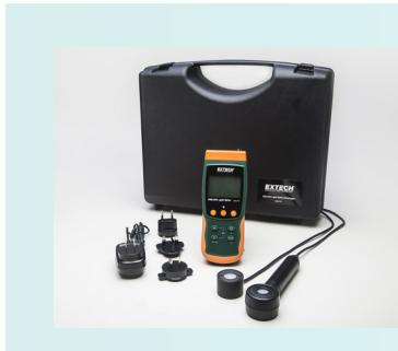
Extech's compact UV Light Meter includes two types of probes: one to measure UVA (long wave 365nm) and the other to measure UVC (short wave 254nm) light sources up to 20mW/cm<sup>2</sup>. The SDL470 date/time stamps and stores files onto an SD card in MS Excel® format to make transferring, storing, and analyzing the data on your PC easier. The unit also has a Type K/J thermocouple input to capture temperature readings (temperature probes not included).
