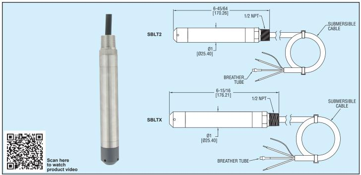
SBLT2 and SBLTX Submersible Level Transmitters are manufactured for years of trouble free service in the harshest applications. Both measure the height of liquid above the position in the tank referenced to atmospheric pressure. The transmitters consist of a piezoresistive sensing element, encased in a 316 SS housing. Bullet nose design protects the diaphragm from damage.
