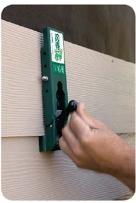
1 At approximately one-third 2 Engage the handle for a snug fit. Don't over-tighten! (See photos A & B)
