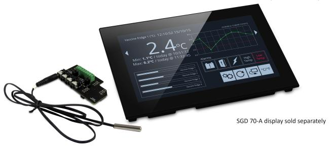
The S70-TP is an accessory to the PanelPilotACE range of compatible displays and panel meters and is compatible with the 7" PanelPilotACE display module (SGD 70-A). The S70-TP mounts on the rear of the SGD 70-A and provides up to four thermistor inputs which can then be utilised within the free PanelPilotACE Design Studio software to measure, display, log and graph temperature readings.
