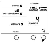
Press this button so the station is ready to have motes join the network
