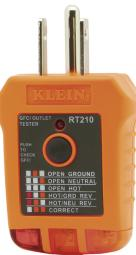
Klein Tools Receptacle Testers are designed to detect the most common wiring problems in standard and GFCI receptacles. A convenient chart on the tester helps determine wiring condition in outlet, based on LED lights results. Conditions indicated: open ground, reverse polarity, open hot, open neutral, hot/ground reversed.
