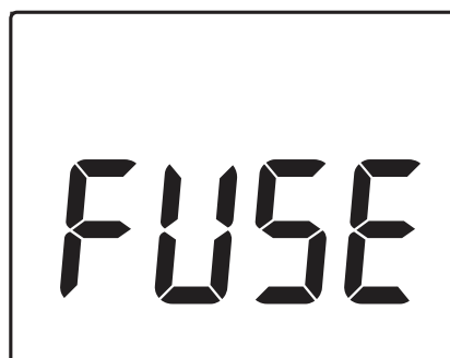
Fuse blown out
