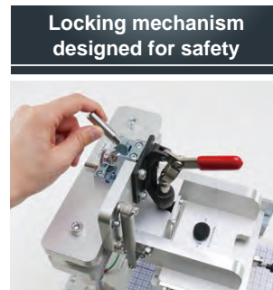
Locking mechanism designed for safety Pull the lock lever toward you to allow the probes to be lowered. This design keeps the probes from being lowered inadvertently.
