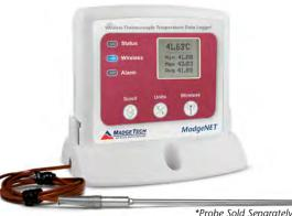
The convenient digital display provides the current reading for both channels. Minimum, maximum and average statistics are also provided for a convenient snap shot of the logged data. For instant, out of range notification, an audible buzzer as well as LED alarm indicator notifies users when the temperature is above or below the user specified alarm. Through the software, email and text message alarms can also be sent.
