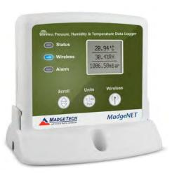
This data logger allows users to select the desired units in which the data is displayed. The RFPRHTemp2000A has a wide range of units available for each channel: °C, °F, °R, K for the temperature channel, %RH, mg/mL, Dew Point for the humidity channel and mbar, PSI, inHg, mmHg, atm, Torr, Pa, m, kPa, MPa for the pressure channel. PSI and mbar are available for display on the LCD screen.
