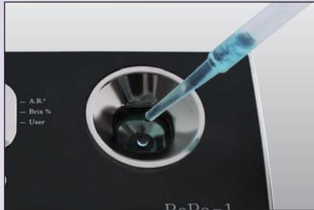
1. Fill the sample stage up to the fill line (approx. 3mL).
