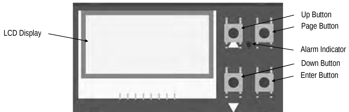
Figure 33: Control Panel for the Comm Box (DIN)
