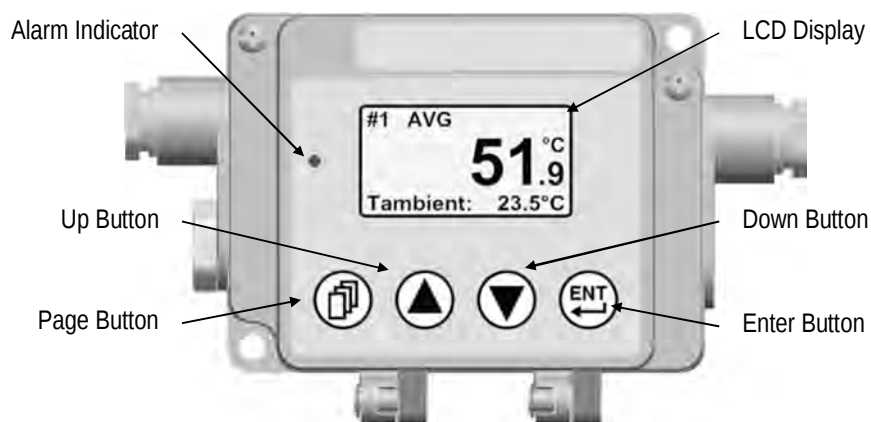
Figure 32: Control Panel for the Comm Box (metal)
