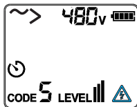
AC voltage (>480V) measurement
