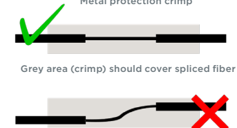
Metal protection crimp
