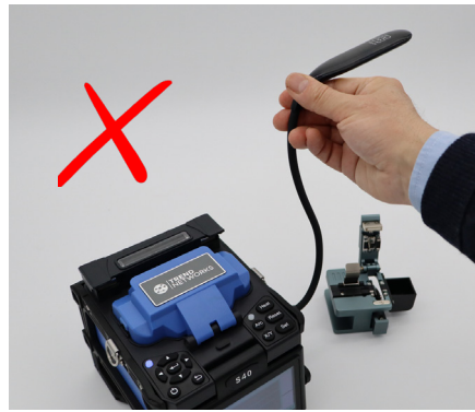
Adjusting LED lamp could cause usb port damage
