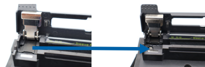
The SoC flap pushes outward to accommodate SoC connector
