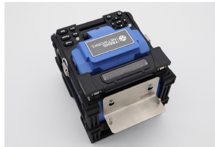
Crimp tool bracket against splicer
