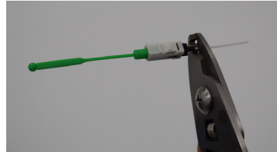
Stripping SoC pigtail by using medium hole on fiber stripper
