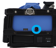
Connect power supply to battery charge port
