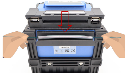
Heat shrink sleeve inside cooling tray
