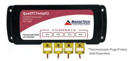
The QuadTCTempV2 is a 4-channel thermocouple data logger with a reading rate of up to 4 Hz. It can measure and record 65,471 readings per channel. To maximize memory capacity, users can enable or disable channels. For easy identification, each channel can be named with up to a ten digit title.
