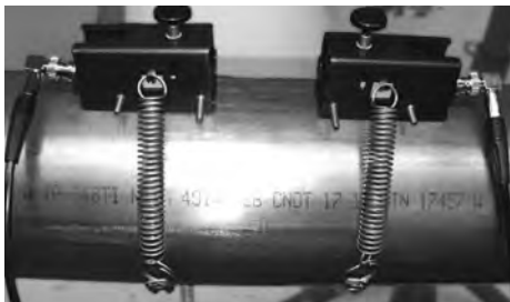
FIGURE 40: V-mode or W-mode with spacer bar
