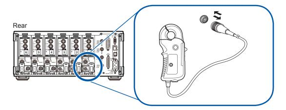
The instrument provides two dedicated terminals for current sensors: Probe1 and Probe2. Use the Probe1 terminal when performing high-precision current measurement with the model 9709 and CT6860 series of AC/DC Current Sensors or the CT6840 series of AC/DC Current Probes. Use the Probe2 terminal when performing wideband current measurement with the 3270 series of Clamp On Probes. Connect each sensor after moving the sliding cover.
