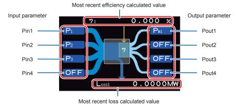
Select the input-side power measured value on the left and the output-side power measured value on the right for each figure on the screen. Up to four inputs and outputs can be selected for each efficiency calculation formula. Efficiency is calculated using the sum of the four.
