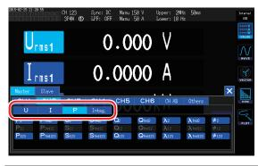
3. Selects the **U**, **I**, **P**, and **Integ.** parameters for CH1 to CH6.
