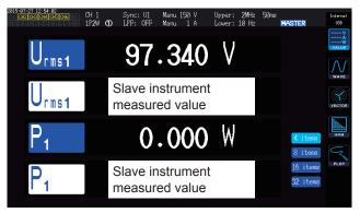
When a measured value from the slave instrument is selected on the CUSTOM screen as a display parameter, the color of the parameter name will be reversed.
