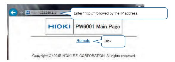
Display of the main page shown in the figure indicates that you have successfully connected to the instrument. Clicking the "Remote" link will open the remote operation page.
