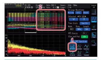
FFT TOP10 measured values can be sent to a computer using the LAN, GP-IB, or RS-232C interface.
