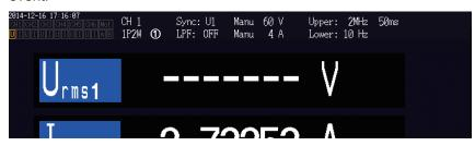
The value display area will be left blank when OFF is selected as the display parameter and when the selected parameter is invalid due to the values of other settings.
