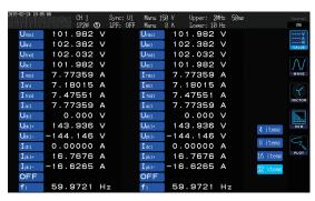
Touch the name of parameter to open the basic measurement parameter selection window. Touch to select the parameters to display.
