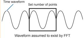
If the number of FFT calculation points does not match the period of the measured waveform, both ends of the waveform in the window will be discontinuous, causing an error known as a leakage error and leading to the detection of FFT analysis results that do not in fact exist.
