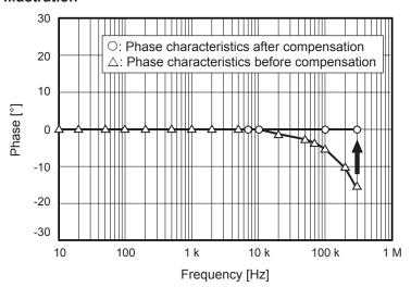
See the table below for information about current sensor phase characteristics. Example settings for the current sensor phase shift function are provided on the following page.
