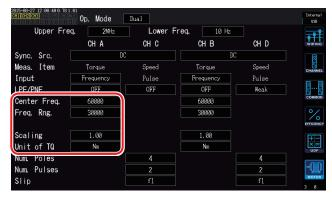
If the **Input** is set to **Frequency**, set the following four parameters based on the sensor: **Center Freq.**, **Freq. Rng.**, **Scaling**, and **Unit of TQ**.
