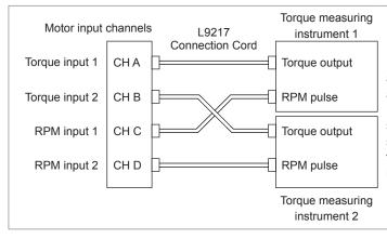
Input one torque signal and RPM signal to CH A and CH C and measure the first motor's power and efficiency. Input the other torque signal and RPM signal to CH B and CH D and measure the second motor's power and efficiency. The torque signals can use analog DC signals or pulse-based frequency input. The RPM signal can use pulse input only.
