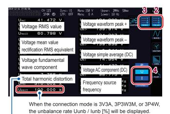
When DC has been selected as the integration mode, the ripple rate will be displayed instead of the total harmonic distortion.
