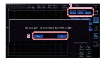
**Under Arrange Waveforms, touch one** of the patterns.
