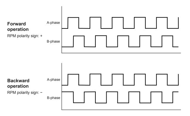
The detected direction of rotation is reflected in the polarity sign that is assigned to RPM measured values as well as to motor power (Pm) measured values.
