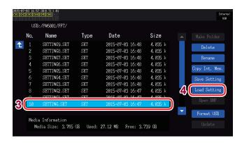
Settings can only be restored when the same options and other characteristics are the same. If the instrument is equipped with different options, you will not be able to restore the settings.
