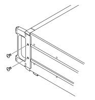
3 Attach the rack-mounting hardware (for both sides) to the instrument with two M4 × 14 mm screws.
