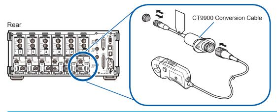
When the CT6865 (rated for 1000 A) is connected with the CT9900 Conversion Cable, it will be recognized by the instrument as a 500 A AC/DC sensor. Use the sensor with the CT ratio set to 2.00.
