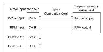
Input the torque signal to CH A and the RPM signal to CH B. Then measure the motor power and motor efficiency. The torque signal can use an analog DC signal or pulse-based frequency input. The RPM signal can use an analog DC signal or pulse input. The torque signal and RPM signal can be input from different sensors.
