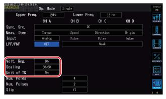
When Torque input is set to Analog, set the following three settings based on the sensor: Volt. Rng. (voltage range), Scaling (scale value), and Unit of TQ (torque unit).
