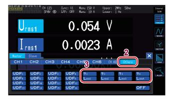
1 Touch the parameter name and select the desired display parameter.
