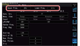
When inputting a pulse signal to the instrument's motor input, set upper and lower limits for the pulse frequency.
