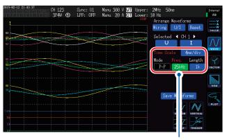
When the settings are changed from those of the displayed waveform, parameters whose waveform and settings differ will be displayed in red.
