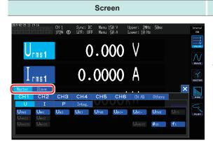
When operating in the two-instrument synchronization function's numerical synchronization mode, selects whether to display Master or Slave first.
