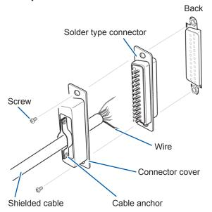
Use the connector included with the instrument to make connections to external control terminals and output terminals (DB-25P-NR, DB19678-2R Japan Aviation Electronics Industry, Ltd.) or equivalent parts.
