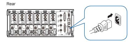
3 Connect the power cord's plug to an outlet.
