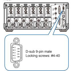
1 Connect the RS-232C cable to the instrument's D-sub 9-pin connector.
