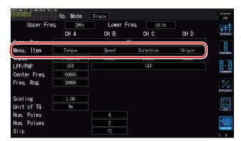
Set how to use CH A through CH D in single motor (Single) mode. You can select from the following four patterns:
