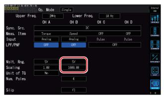
If the Input is set to Analog, set the Volt. Rng. (voltage range) and Scaling (scale value) based on the rotation signal.
