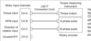
Input the torque signal to CH A, the A-phase pulse signal to CH B, and the B-phase pulse signal to CH C. Then measure the motor power and motor efficiency while viewing the direction of the motor's rotation based on the phase difference between the A-phase pulse and the B-phase pulse. The torque signal can use an analog DC signal or pulse-based frequency input.
