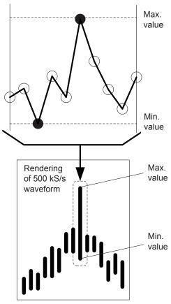
When a 5 MS/s waveform is subject to peak-peak compression to yield a 500 kS/s waveform
