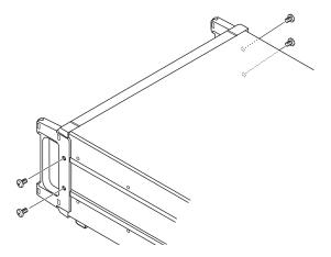
3 Attach the rack-mounting hardware (left-/right-side hardware) to the instrument with two M4 × 14 mm screws.
