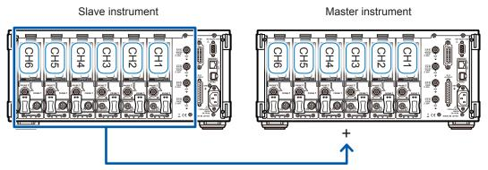
Transmission of measured values for basic measurement parameters
