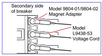
Connect the magnetic part of the 9804-01 or 9804-02 tip to the screws on the secondary side of the breaker.
