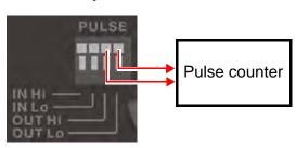
A pulse signal is output each time active energy consumption (WP+) exceeds the pulse output rate during recording and measurement. The output rate can be set from 1 Wh to 1,000 kWh.
