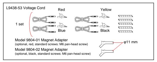
Voltage cords used by wiring type
