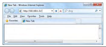
If the main page is displayed as shown below, you have successfully connected to the instrument:
