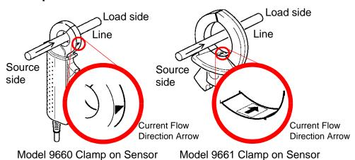
Attach the clamp around only one conductor. Single-phase (2-wire) or three-phase (3-wire) cables clamped together will not produce any reading.
