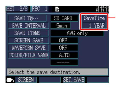
Data storage time Since the instrument can perform recording and measurement for a maximum of one year, the maximum data storage time is one year.
