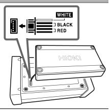
With the battery case facing down, fit it into the recessed area on the instrument.
