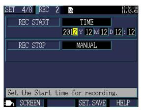
3 Change the setting with the \( \omega / \omega \) cursor keys and then accept the new value with the ()[ENTER] key. Change other settings as necessary.
