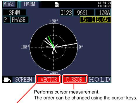
The display can be changed from the normal bar graph to a vector graph when the display parameter is set to the active power phase angle display. Length is displayed using the LOG axis.
