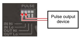
Input a pulse signal from an external source. After configuring scaling (coefficient), sub-unit, and unit (five byte characters) settings, you can convert and measure an input pulse signal. After recording and measurement are started, pulse input values are saved for each save interval.
