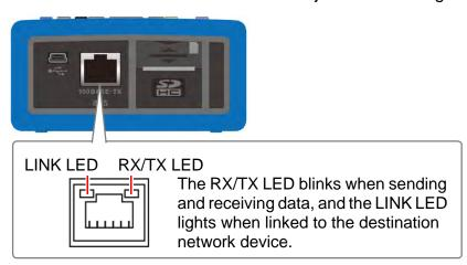
When connecting the instrument to an existing network (when connecting the instrument to a hub)
