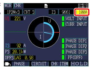
ment, making accurate measurement impossible. Conversely, if the range is too high, the error will be too large, making accurate measurement impossible. Set the current range based on the maximum load current that is anticipated during the measurement interval.
