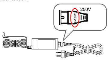
Connect the Z1006 AC Adapter to the instrument and plug it into an outlet as follows:
