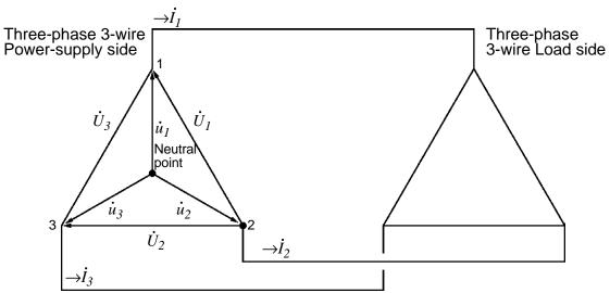
An artificial circuit of a three-phase 3-wire line
