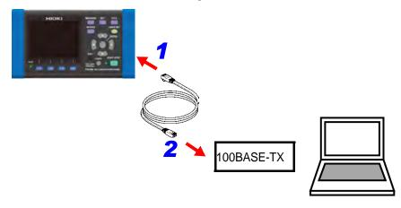
NOTE Since the instrument provides functionality for automatically detecting whether a straight or cross cable is being used, a straight cable may also be used. If you are unable to establish communications with the computer, try a cross conversion cable (9642 accessory).
