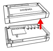
Remove the single screw holding the 6 board in place and remove the board.
