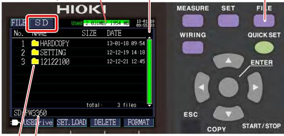
Displays the current display location. In this case, the screen is displaying the PW3360 folder on the SD memory card.
