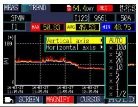
3 Select the desired zoom factor with the cursor keys and press the [ENTER] key.
