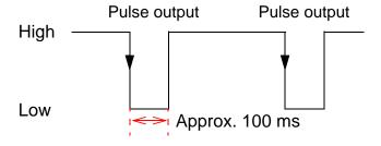
The pulse output terminal is isolated from the instrument's internal circuitry. When using pulse output, connect the "PULSE OUT Hi" terminal to an external power supply using a pull-up resistor as shown in the following example external circuit:
