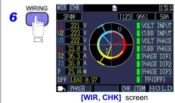
Set the current range. (p. 61) Check the wirings. (p. 63)
