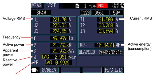
Selects between power factor PF (RMS calculation) and displacement power factor DPF (fundamental wave calculation) with settings.
