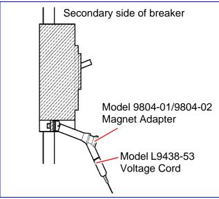
The weight of the voltage cords may prevent you from making a perpendicular connection to the Model 9804-01 or 9804-02 Magnet Adapter. In this case, connect each cords so that it is hanging off the adapter in a manner that balances its weight. Check the voltage values to verify that the connections have been made securely.
