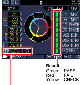
The power factor is displayed as DPF (displacement power factor) on the Connection Confirmation screen, regardless of the [PF/Q/S CALC] setting.
