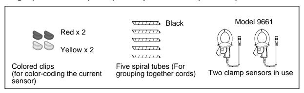
Attached color clips of the same color around the connector and sensor sides of the clamp sensor cable.
