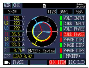
5 Move the cursor to the item that has been tagged as red (FAIL) or yellow (CHECK) and press the [ENTER] key.
