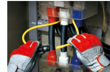
AC FLEXIBLE CURRENT SENSOR CT9667-01, -02 (Sold separately)
