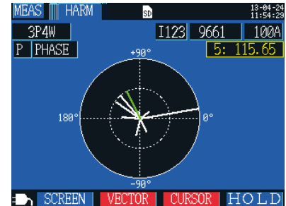
Harmonic power phase angle graph screen
