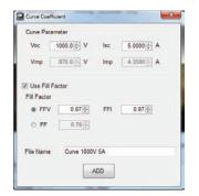
Automatically generate the I-V curve of a solar array in the software by specifying open circuit voltage (Voc), short circuit current (Isc), maximum power voltage (Vmp), and maximum power current (Imp) along with fill factor parameters.
