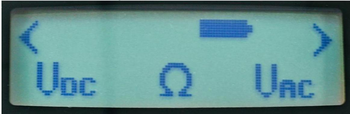
Connect the Pro50™ to the zone or item you wish to test. Press F1 for DC Voltage, F2 for resistance ohms, or F3 for AC Voltage. The Pro50™ has auto-range capability, meaning that the expected range is not required to be entered into the Pro50™.
