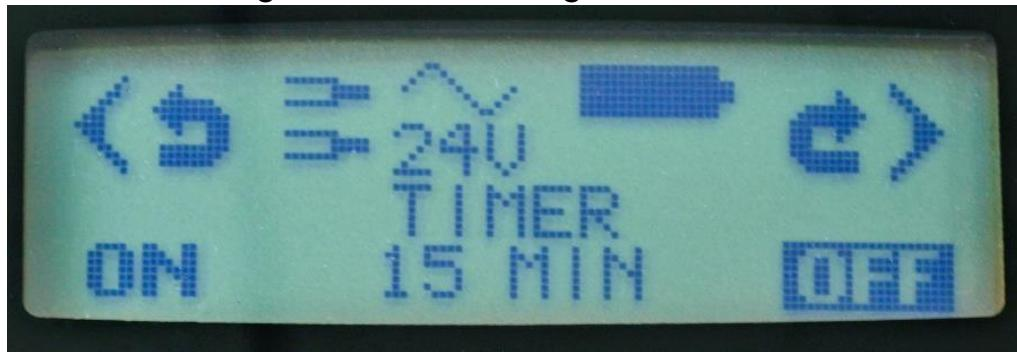
4. Press F1 ON to power the 2-wire cable. This will provide power to the two-wire cable for 15 minutes before timing out. Press F2 if you'd like to change the timeout from 15 minutes to 30 minutes.
