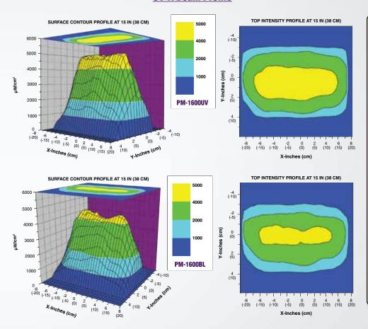
PowerMAX™ 365 Series UV-A LED panel flood lamps are also available in two standard-intensity models that are designed for NDT inspection applications requiring limited UV-A output. Both versions address aerospace industry concerns.
