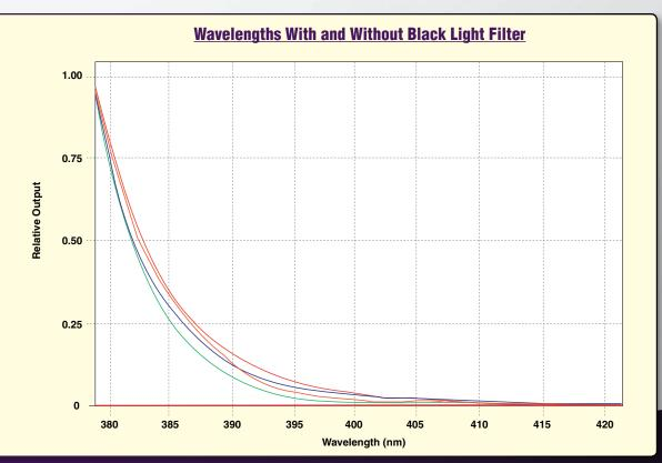
As the wavelength of the PowerMAX™ 365 moves into the visible light range, the black light filter significantly reduces the output of the lamp at 400 nm.
