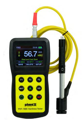
State of the art, digital tester is designed to test the hardness of large hard metal parts. Clean crisp display shows the incredible functions that can only be found on this new model such as auto-probe detection, auto direction detector, single and multi-point calibration make the new 1900 the most versatile portable hardness tester in the industry. Blazing fast test speeds coupled with memory and output, this unit is a must have for virtually any work shop.
