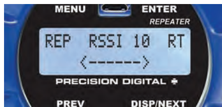
▲ Close-up of PDW30-RNA Repeater Display
