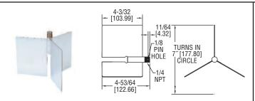
PDL-1. 316 SS three vane paddle for light weight materials with a minimum bulk density of 5 lb/ft3 (80 kg/m3).
