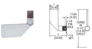
PDL-4. 316 SS single vane paddle for heavy weight materials with a minimum bulk density of 70 lb/ft3 (1122 kg/m3). Fits through 1-1/4" coupling eliminating the need for a mounting flange.
