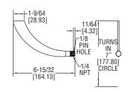
PDL-3. 316 SS single vane paddle for medium weight materials with a minimum bulk density of 30 lb/ft<sup>3</sup> (481 kg/m<sup>3</sup>). Fits through a 1-1/4" coupling eliminating the need for a mounting flange.
