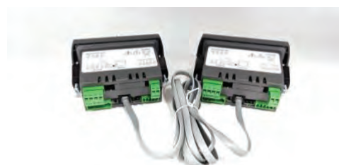
Figure 17. Trident Copy Cable Connecting Two Meters
