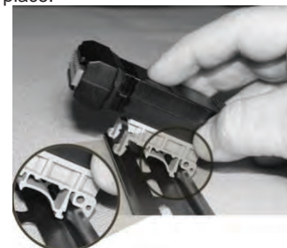
Figure 7. Snapping the Module to the DIN Rail
