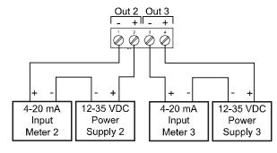
Figure 4. Dual Analog Output Module Connections
