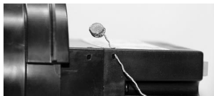
Figure 4: Wire Loop through Rear Case Pass-Through
