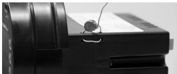
Figure 6: Close and Crimp Seal Wire Security Loop
