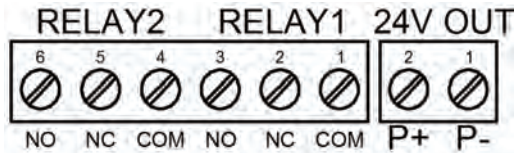
Figure 12. Relay & 24 V Output Connections
