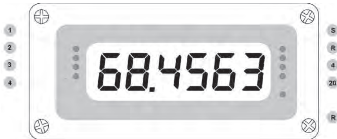
Figure 25. Front Panel LED Indicator Locations
