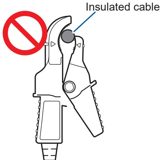
The sensor is affixed to the insulated cable at an angle.
