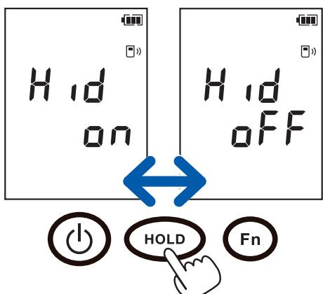
The HID function can be selected when the wireless communication function is enabled. Simultaneously pressing and holding the **HOLD** and **Fn** keys toggles the wireless communications function on and off. The display will show the
