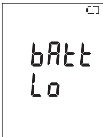
When the indicator shows no remaining battery power (the icon is blinking), the string **[bAtt Lo]** will be shown for 2 s, and the instrument will shut down.
