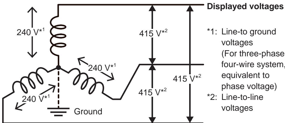
The 400 V line depicted in the figure has line-to-line voltages each of which is 415 V yet has line-to-ground voltages each of which is approximately 240 V. You can use a measuring instrument whose the input rating of a line-to-ground voltage is 300 V to measure this circuit
