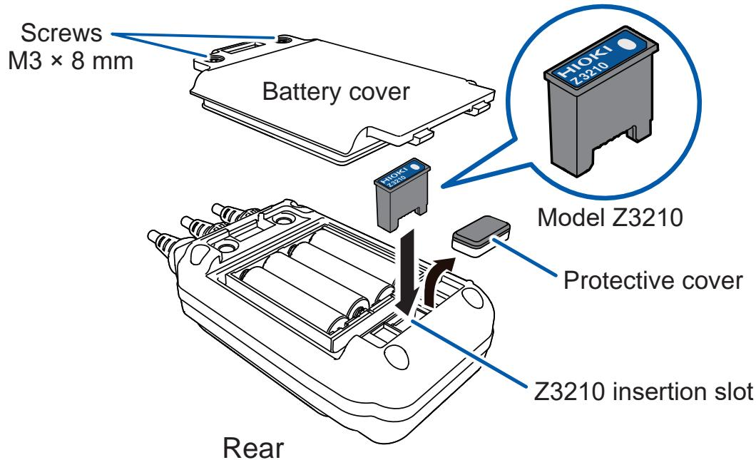
To maintain the dust resistance and water resistance, put the protective cover on the Z3210 insertion slot regardless of the presence or absence of the Z3210.
