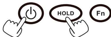
Turn on the instrument while holding down the **Fn** key.
