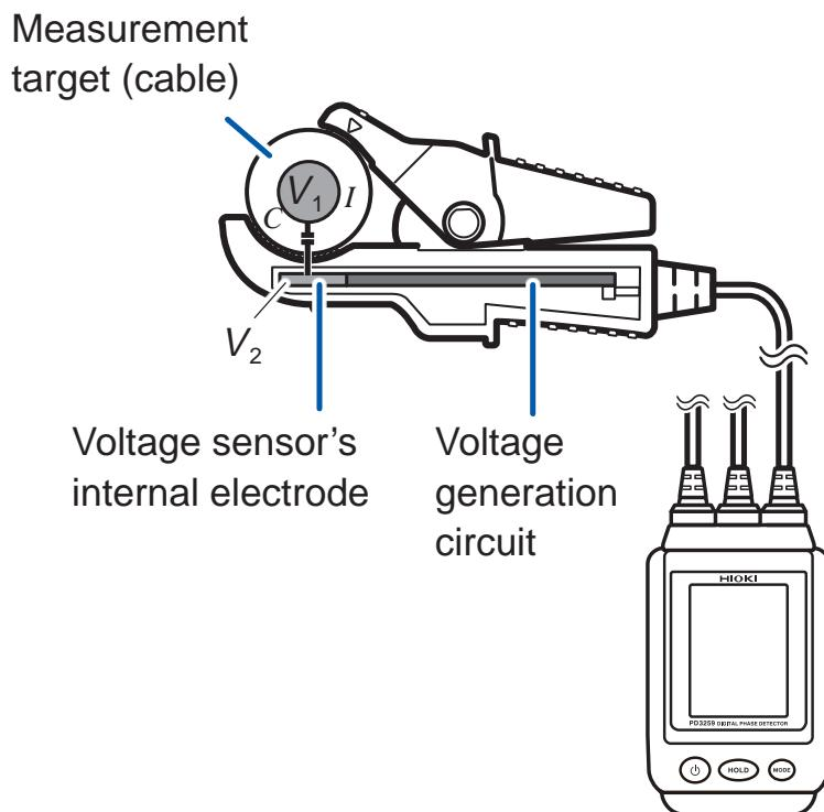
$V_2$  is controlled so that  $I = 0$ .
