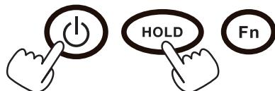
Turn on the instrument while holding down the **HOLD** key.
