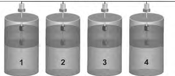
Tanks with Multivariable Level Transmitters
