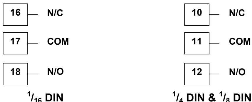
Figure 27. Option Slot 3 - Relay Module
