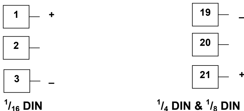
Figure 19. Option Slot 1 - SSR Driver Module
