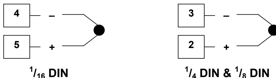
Figure 15. Thermocouple Input Connections
