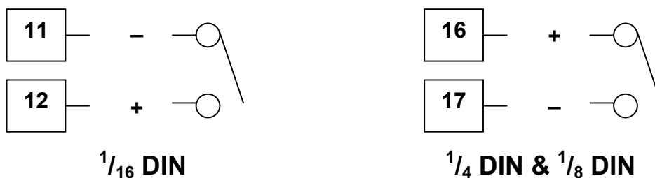
Figure 33. Option Slot A – Digital Input Module
