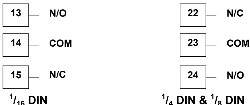
Figure 22. Option Slot 2 - Relay Module
