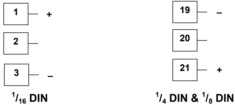
Figure 21. Option Slot 1 - Linear Voltage & mADC Module
