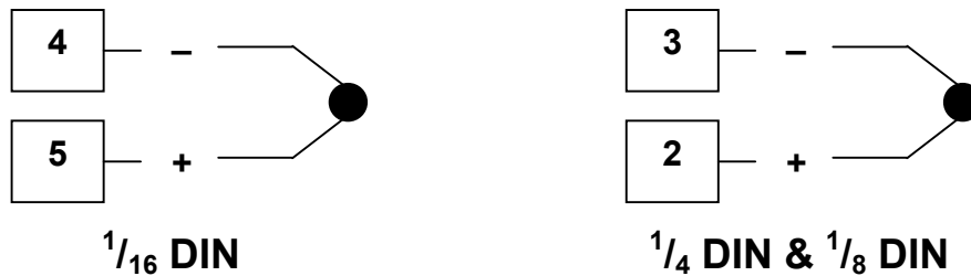
Figure 15. Thermocouple Input Connections
