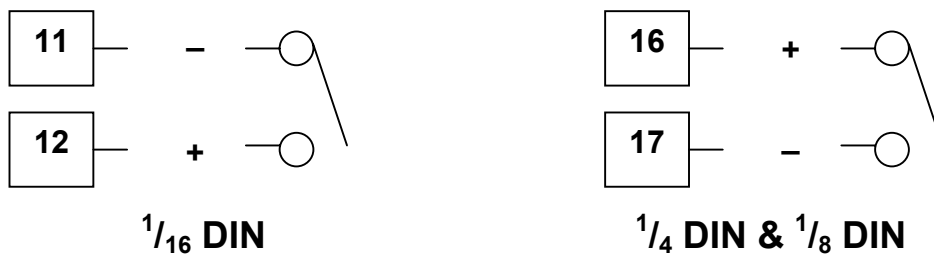
Figure 33. Option Slot A – Digital Input Module
