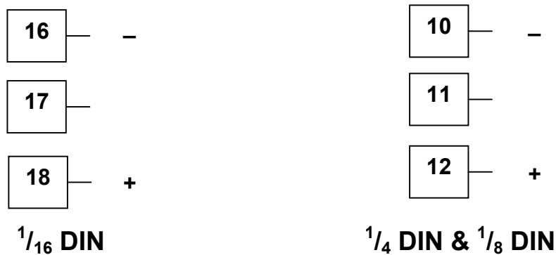
Figure 28. Option Slot 3 - SSR Driver Module
