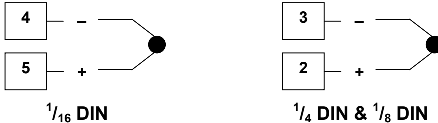
Figure 15. Thermocouple Input Connections
