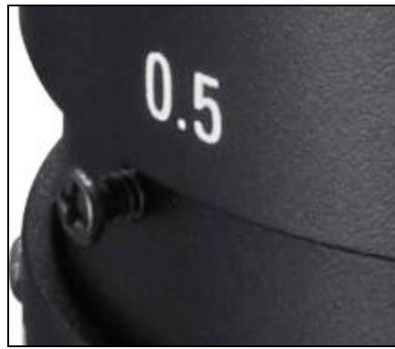
Figure 15: Fixing the focus for PI 05M/ 08M/ 1M
